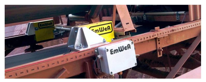
The weighing assembly consists of the modular IDEA-LB weighing frame, and the speed sensor WI520 or ZA-11. It also utilizes a modern electronic integrator.
